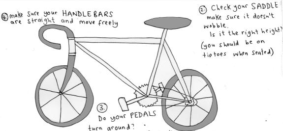
5) Check both BRAKES are Working and Cables aren't Frayed or rusty. turn around? ... make sure your cranks are fixed tightly
